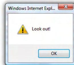
Figure 4.7 By default, exceptions that occur during asynchronous postbacks are displayed in alert dialogs.
